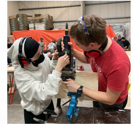
Using domino's and woodglue to connect two big pieces
