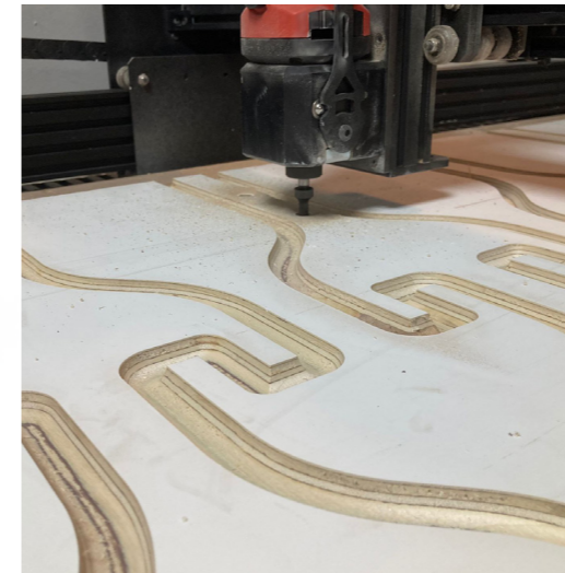
CNC machining the wooden spiders
