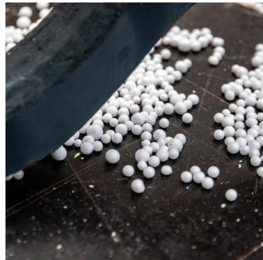
Filling the storage with EPS particles
