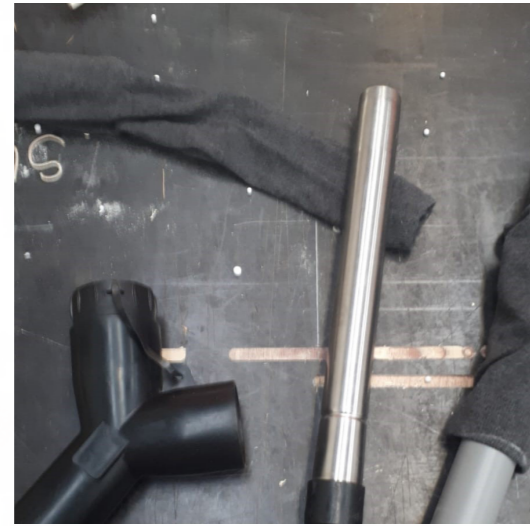
After realizing the need for two vacuum cleaners because of the two separate storages, a PVC divider piece was used. Also, the hole for the vacuum cleaner hose wasn't airtight enough and the textile was blocking the air too much, so a sock was used as a filter instead
