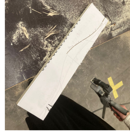
Sawing the individual pieces of the wooden mould with a jigsaw using the printed template
