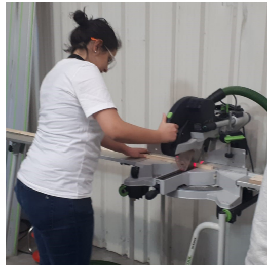
Sawing the wooden spacers for inbetween the three layers of Vivak
