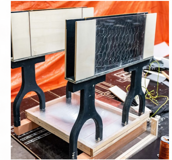
After some discussion it was decided to revert the storages to their original color and to add a perspex panel to be able to look into the storage. During the test, immediately some problems occurred, which are described in the next part
